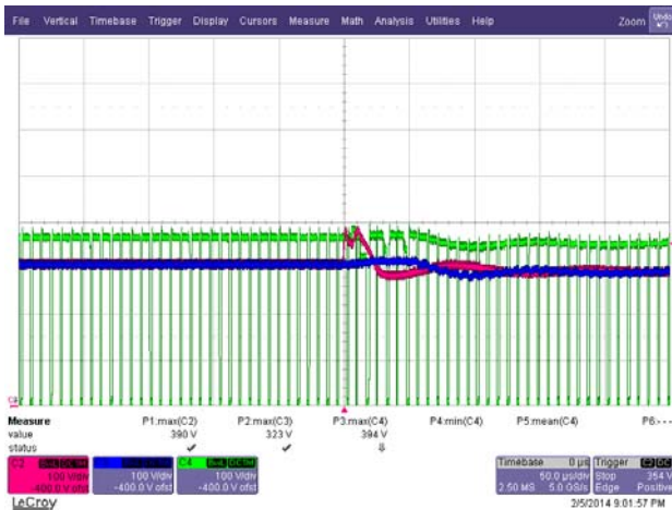
Figure 48 – 230 VAC / 50 Hz, Load: 72 V LED String. Ch2: V BR , 100 V / div. Ch3: V BULK , 100 V / div. Ch4: V DRAIN , 100 V / div. Time Scale: 50 µs / div..
