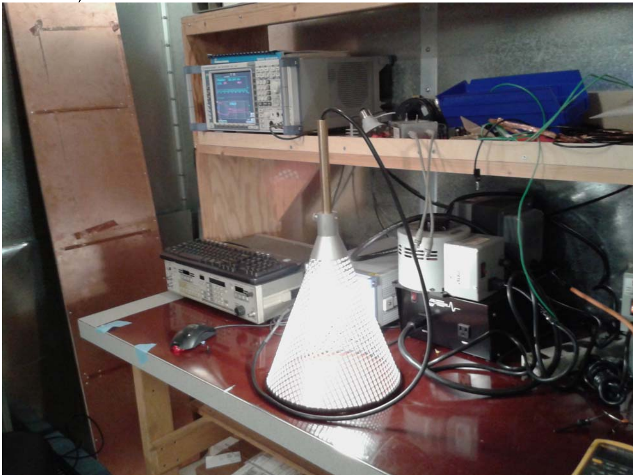
Figure 58 – Conducted Emissions Measurement Set-up.
