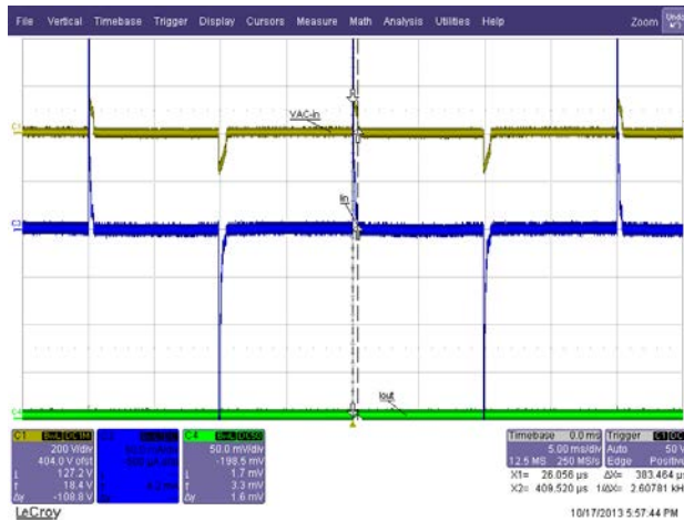
Figure 104 – Minimum Conduction from Distorted AC Line 230 V / 50 Hz. Ch1: V_{IN} ; 200 V / div. Ch3: I_{IN} ; 50 mA / div. Ch4: I_{OUT} ; 50 mA / div. Time Scale: 5 ms / div.
