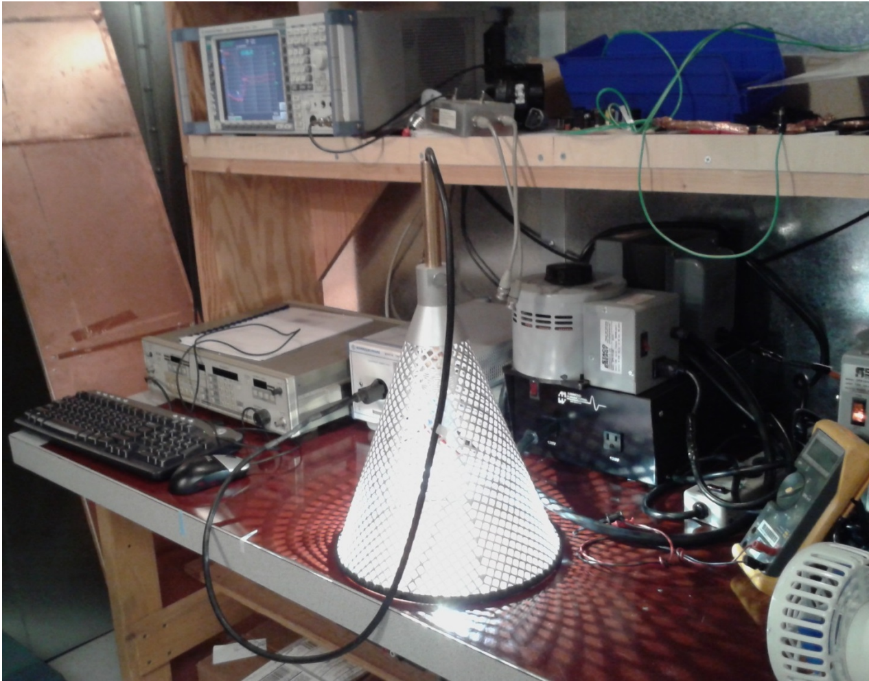
Figure 223 – The Retrofit Lamp was Verified in a Conical Cone as per EN55015.
