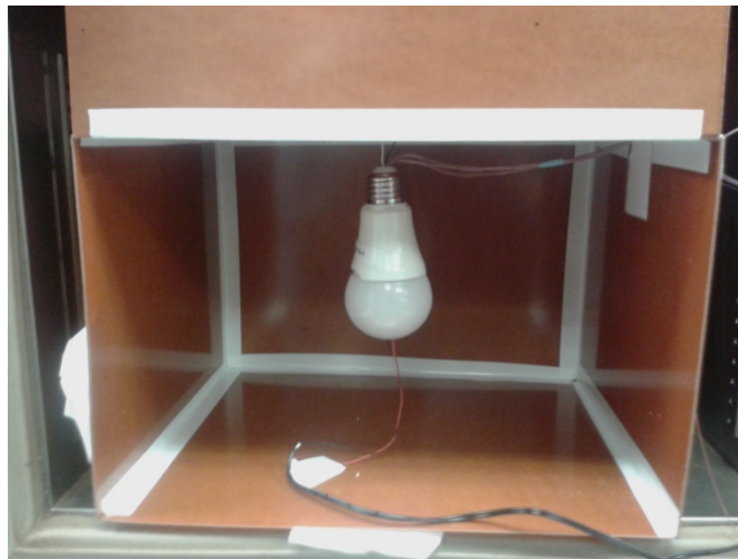
Figure 18 – Thermal Unit Thermocouple Measurement Set-up.
