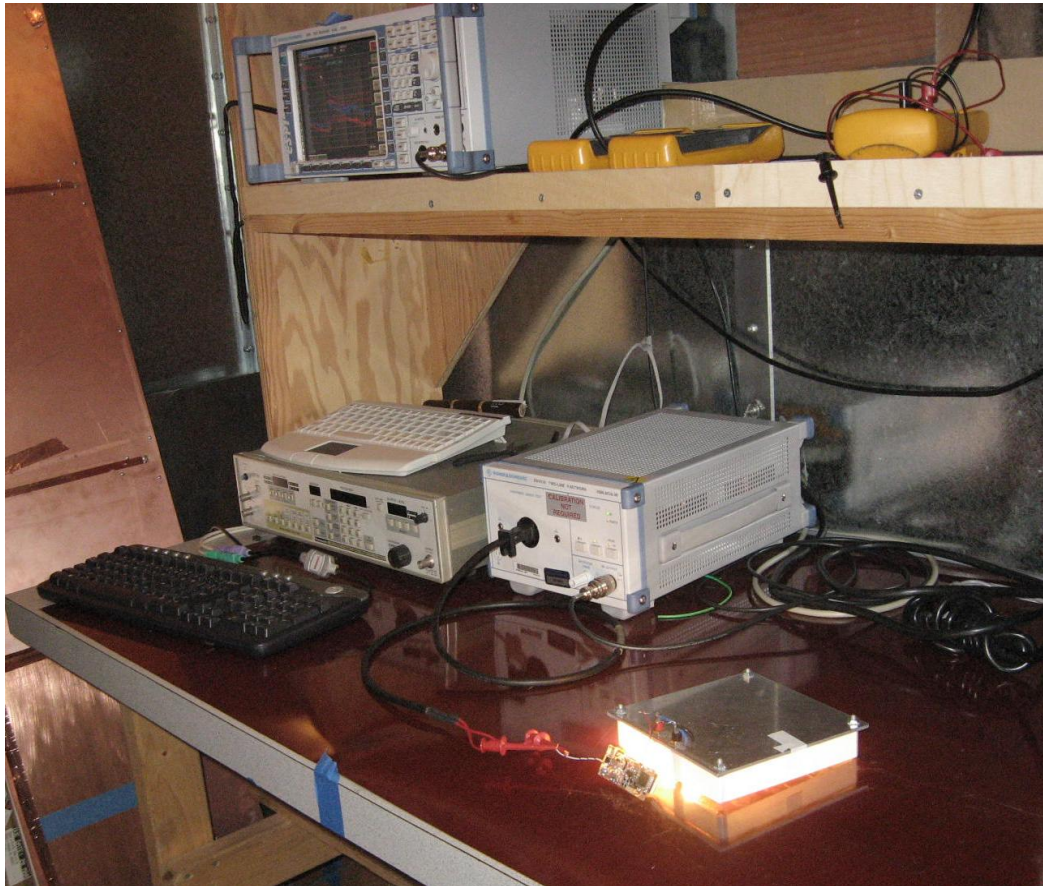
Figure 48 – Conducted Emissions Measurement Set-up.
