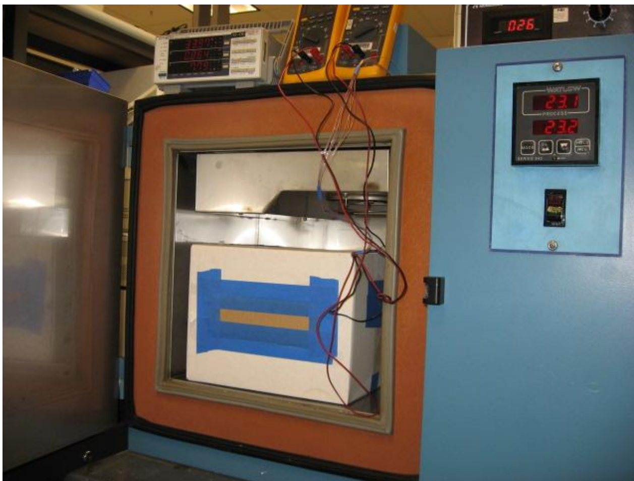
Figure 18 – Thermal Chamber Set-up Showing Box Used to Prevent Airflow Over UUT.
