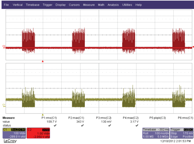
Figure 55 – 90 VAC, 60 Hz Output Short Condition. Upper: I_{DRAIN} , 1 A / div. Lower: V_{DRAIN} , 100 V, 100 ms / div.
